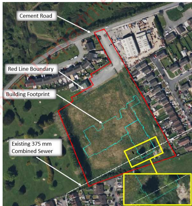
Figure 19: Existing Combined Sewer Overlap with Building Footprint
