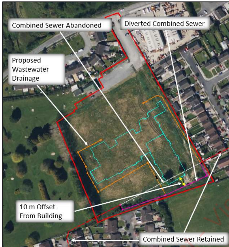
Figure 20: Diversion of the Existing Combined Sewer
