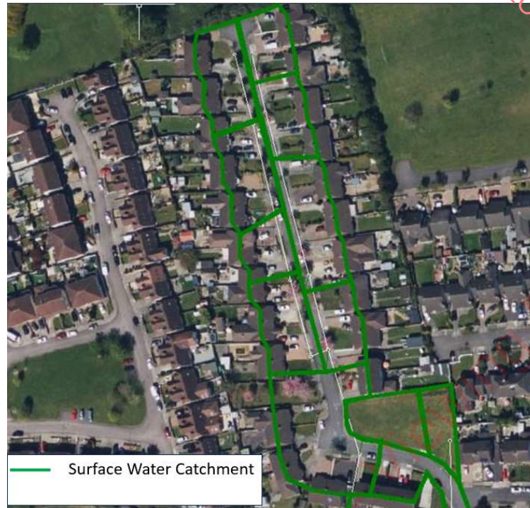
Figure 18b: Catchments Considered in the Existing Network
